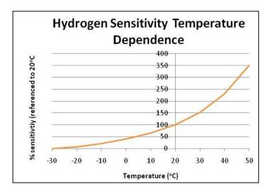
This graph shows hydrogen sensitivity of the CO sensor at different temperatures. Though the graph shows strong temperature dependence of the sensor at temperatures, at low temperatures the hydrogen interference can practically ignored. Where hydrogen sensitivity is <2% of measured gas at 900ppm H2 in 900ppm CO at 10°C and less than 4% at 20°C as well as only 6% at 30°C.
