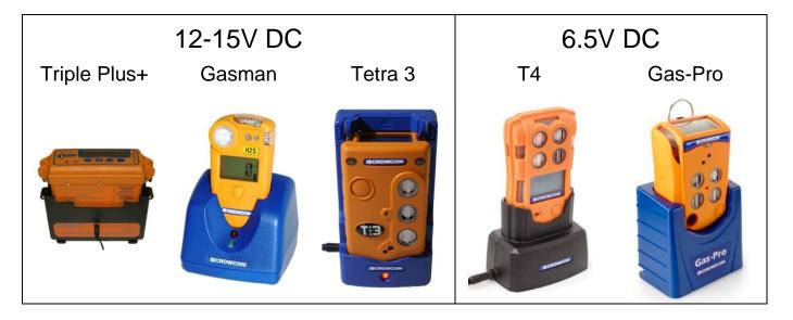
**Triple Plus+, Gasman** and **Tetra 3** charger cradles use a **15V** universal power adapter (product code C03580). A vehicle power adapter is also available which can be used with these charger cradles, and supplies 12V (product code C01296).
