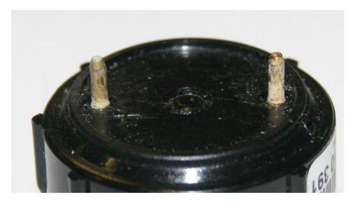
If leakage has occurred the contamination of the sensor pins and PCB sockets increases resistance resulting in reduced sensor signal (and subsequent calibration failure). It may be possible to restore performance by cleaning the sensor pins and sockets using iso-propyl alcohol and a soft brush
