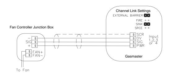
Connect the ESU fan controller to the **Vortex** control panel as shown. Refer to the Appendix C of this manual for details on how to configure the input channel.
