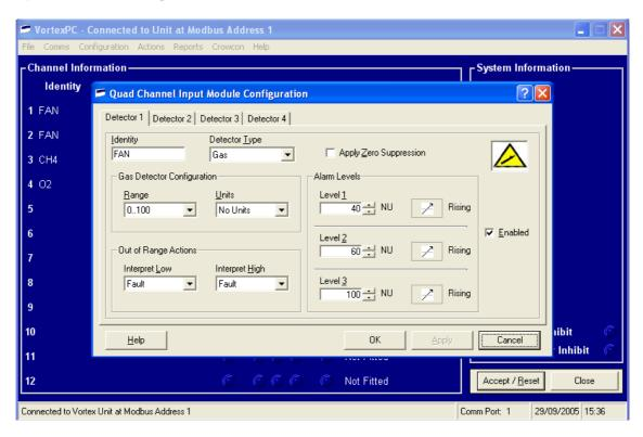
b) Fault ('Fan Stopped or Disconnected') relay configuration: the selected Fault relay must be set with a 3 second off delay. Level 1 and Level 2 'Fan Slow' and 'Fan Stalling' alarms can be set as latching or non-latching as required.
